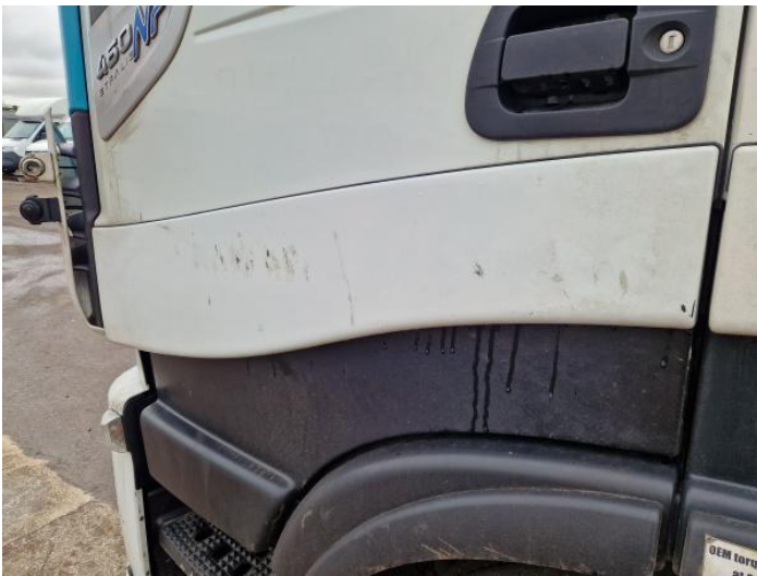
5: Door nsf Scratched Over 25mm Thru Paint
