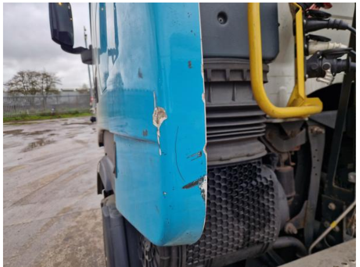
6: Spoiler Rear Broken Replace
