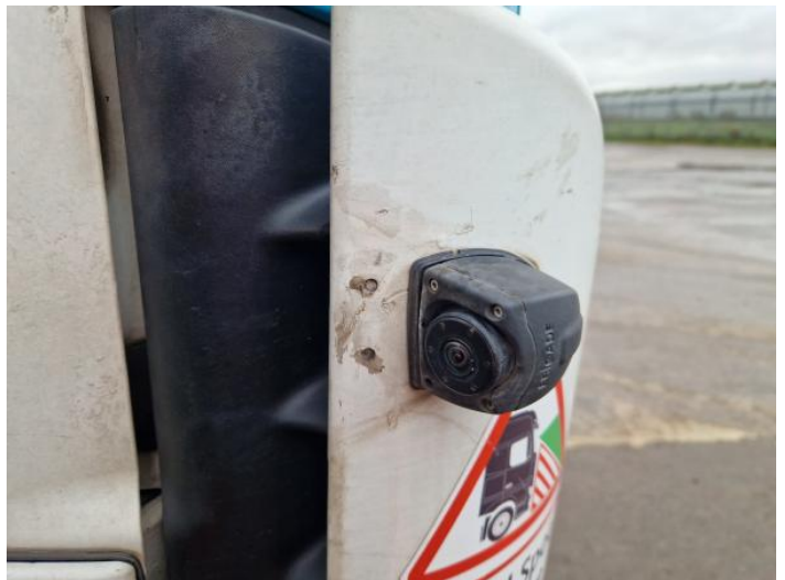
2: Wing osf Poor Previous Repair Poor Paint
