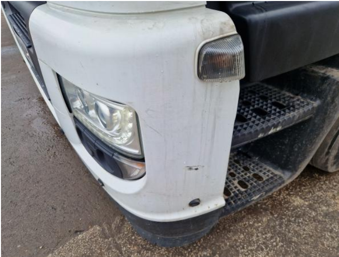
3: Bumper Front Scratched Over 100mm Thru Paint
